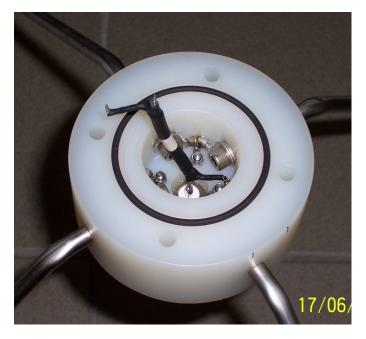
and the finally assembled antenna with quite some silicone grease around the gasket to make it watertight.
