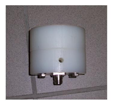
The N-connector is in place and here we see a hole where a radial will be mounted later. Ah yes, I filled up the radial tubes on the body side with silicone compound. The radiator on both sides. All we want to avoid later is getting moisture into the body.
